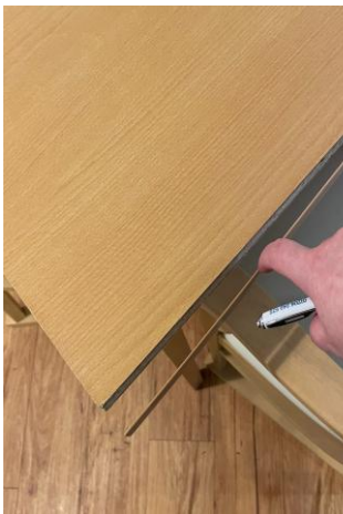
Hazard: table edging hanging off
