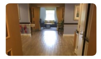
However, although most floors and surfaces have non-reflective / low - sheen treatments, one corridor floor which led to a pleasant seating area (focussed by a large, sun-lit window) displayed a highly reflective sheen which could be perceived as 'water' or 'ice 'to a person with dementia and could inadvertently induce a state of anxiety and/or confusion if not addressed.
